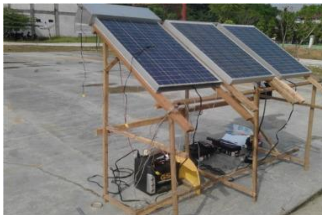
Figure I-15: Outdoor experimental setup consisting of a reference PV, PV-PCM1 and PV-PCM2 installed
