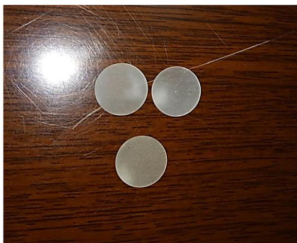
**Figure III.1:** KBr discs prepared for the FTIR
