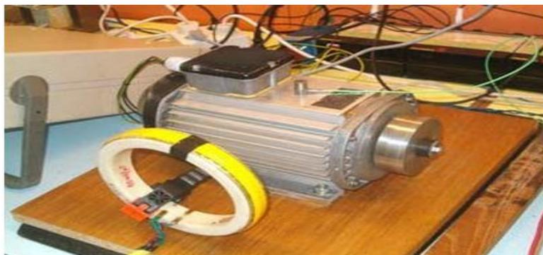
Figure.II.9.Mesure du flux radial [ALL10].
