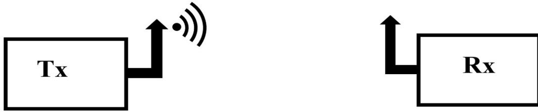
Figure 1.10: SISO - Single Input Single Output
