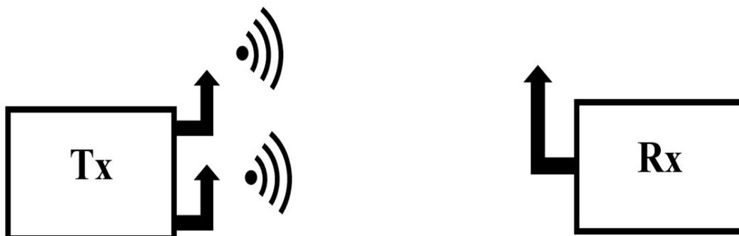
Figure 1.12: MISO - Multiple Input Single Output
