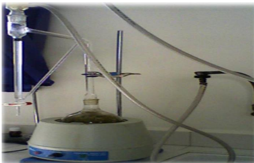
Figure 09: appareil d'hydrodistillation (Clevenger) (Pibiri M., 2006).
