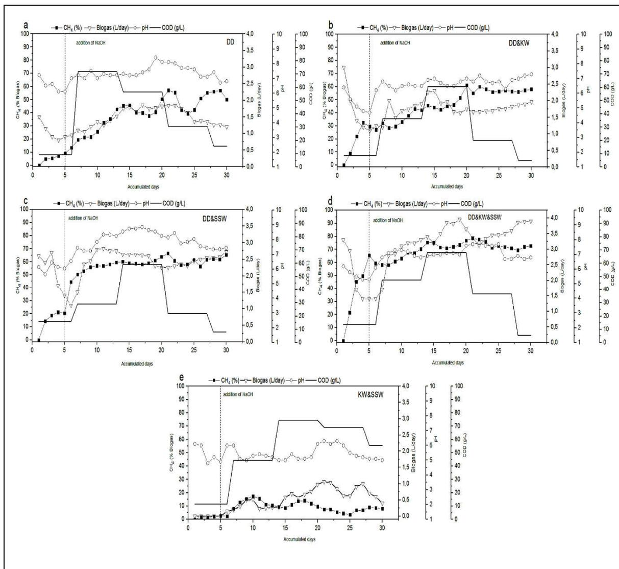
**Fig.3.** Profile of biogas, methane production, pH and COD during anaerobic digestion process of (a) R1, (b) R2, (c) R3, (d) R4 and (e)
