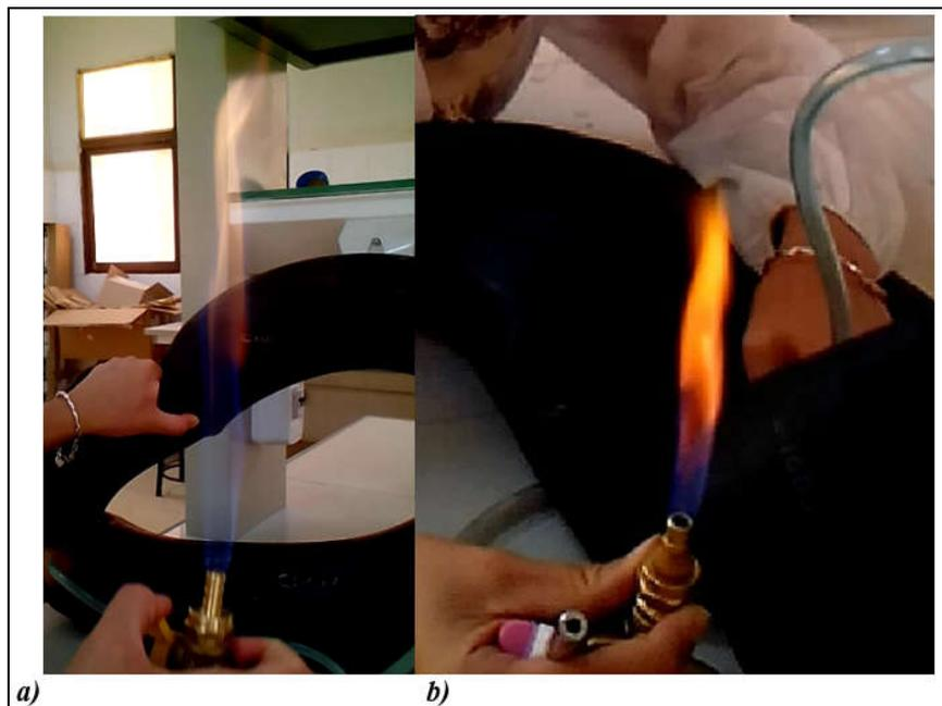
**Fig.4.** Flammability test for R3 and R4, respectively, on the 8th day of incubation
