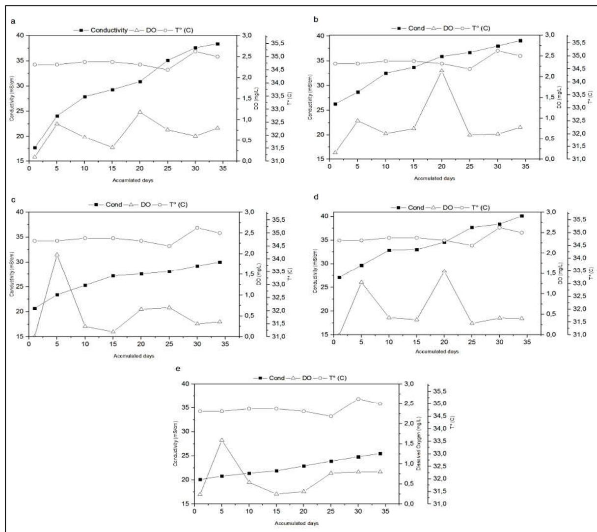
**Fig.2.** Physicochemical parameters influence during anaerobic digestion process on (a) R1, (b) R2, (c) R3, (d) R4 and (e)
