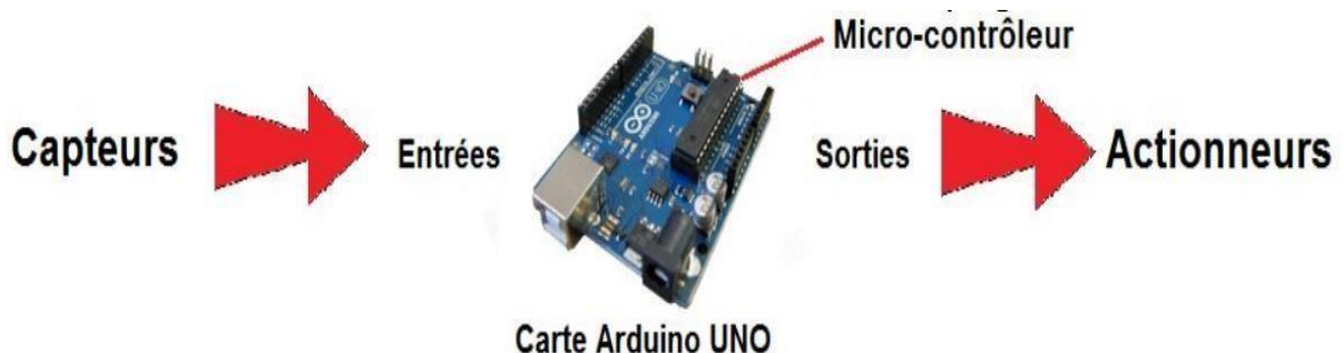
Figure II. 1 : Architecture de la carte arduino UNO
