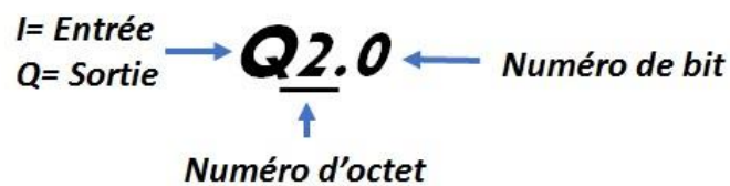
Figure III-2: Adressage Siemens SIMATIC S7
