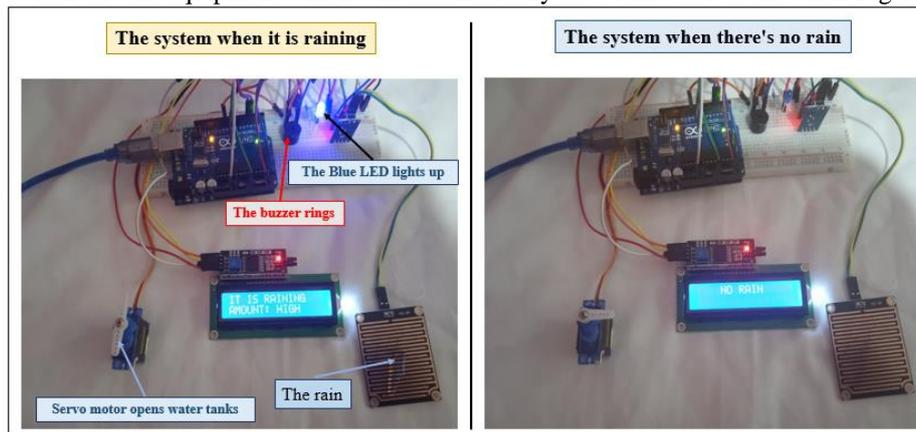
Fig. 11. Rain detection system.
