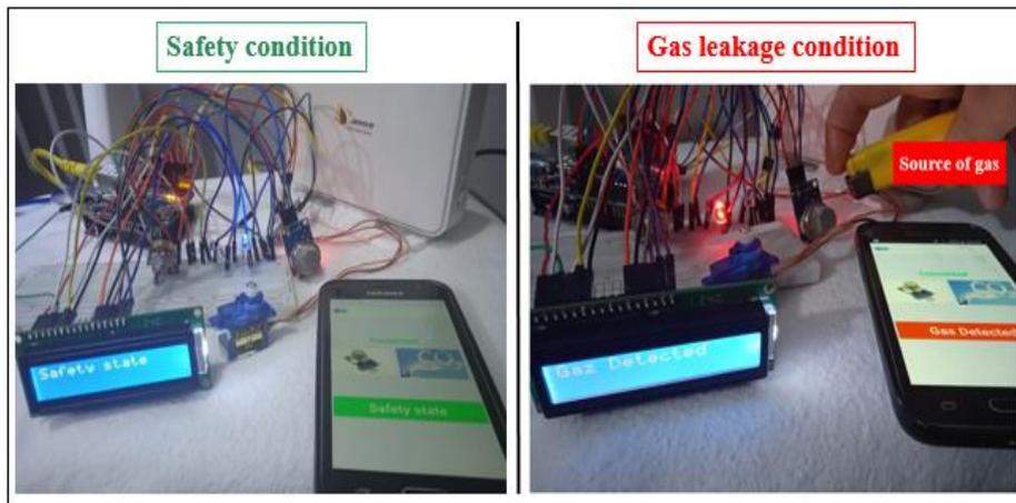
**Fig. 3.** Gas leak detection system.
