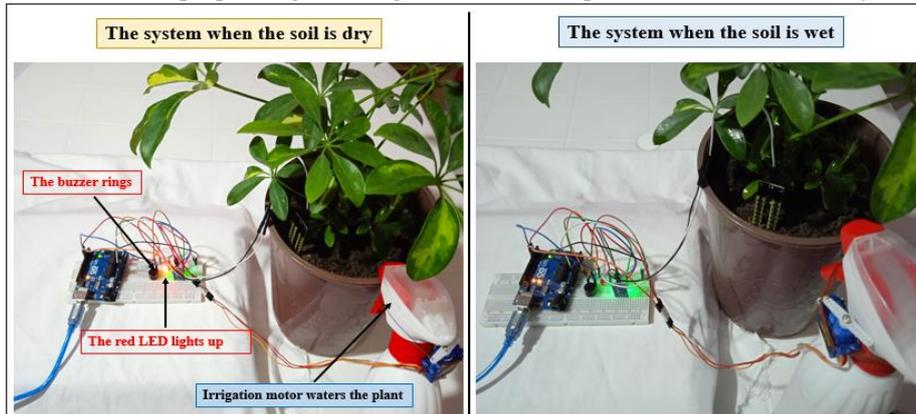
Fig. 10. Garden irrigation automation system.
