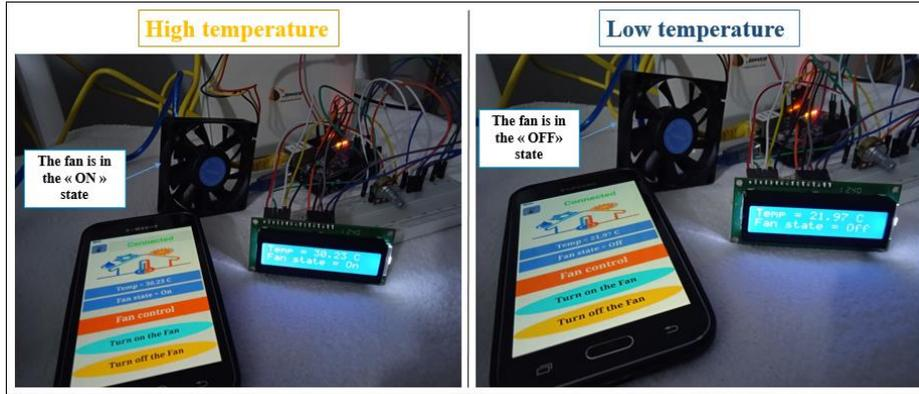
Fig. 9. Temperature monitoring and fan control system.
