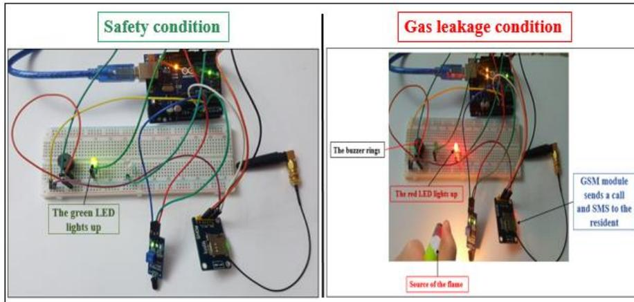
**Fig. 5.** Fire alarm system.
